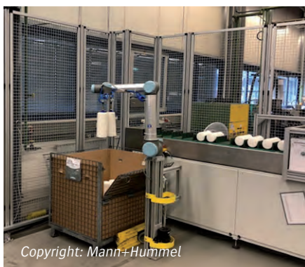
Taking out the filters of a grid box and placing them on a timed conveyor belt in the exact position: Mann+Hummel's new "employee" does not get tired and does not make mistakes
