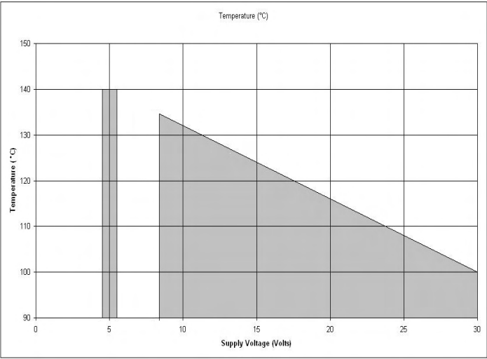
FIG 3 MAX OPERATING TEMPERATURE DERATING
