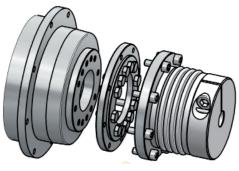
For the connection of the KPE series to the ISO-9409 interface an intermediate flange is required. For the fastening of the coupling flange, the scews are situated above the outer diameter of the bellows. For the mounting of the output side EASY-clamping hub drive shaft connection, a radial bore is required. Installation space depth for coupling mounting must be at least A = X + L.
