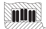
YSKD Series QSKD Series Internal - Heavy Duty 1 set = 3 individual rings (1 rings rotate with bore & 2 rings rotate with shaft)
