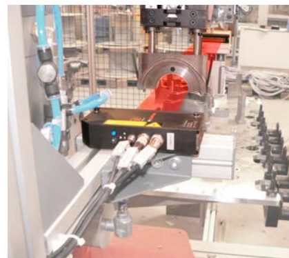
Bearing shell detection in automotive manufacturing
