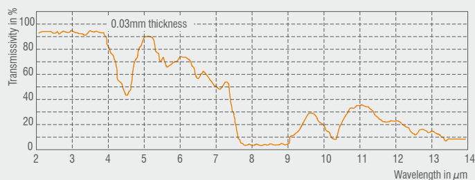
Spectral transmissivity of plastic layers made of polyester
