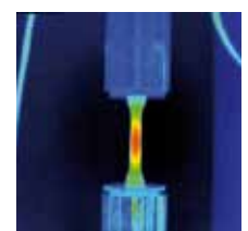
Stress field measurement
