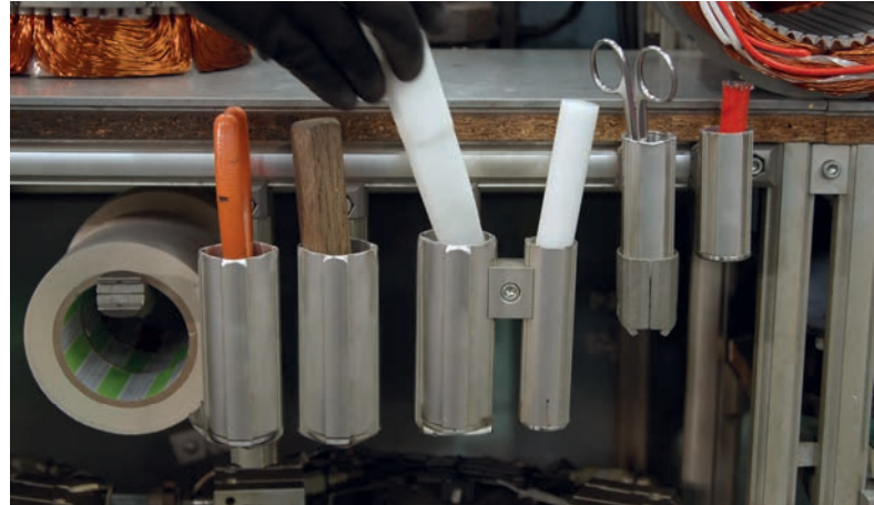
The work time was measured by attaching sensors to the tool holders
