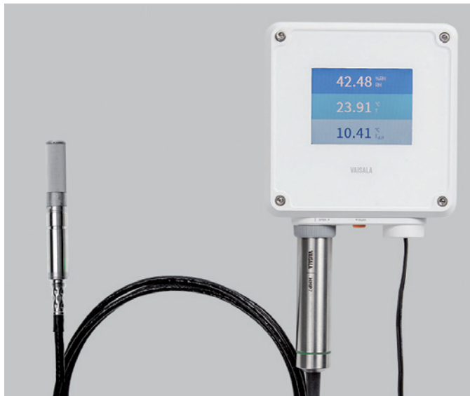
Vaisala HUMICAP® HMP7 is an interchangeable humidity and temperature probe with Modbus RTU output, and is compatible with Vaisala Indigo series transmitters. The probe includes the latest-generation Vaisala HUMICAP® R2 sensor, which provides excellent accuracy and long-term stability and can tolerate temperatures of up to 180°C
