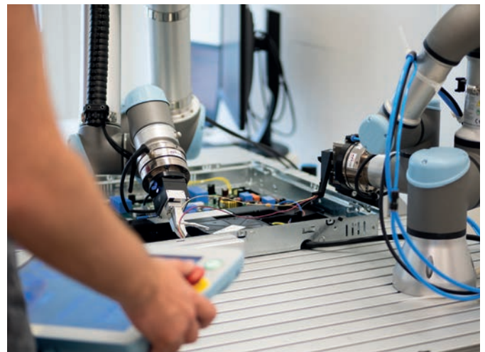
Advanced robotics applications such as the assembly of flexible cables pose a major challenge for classical robot programming
