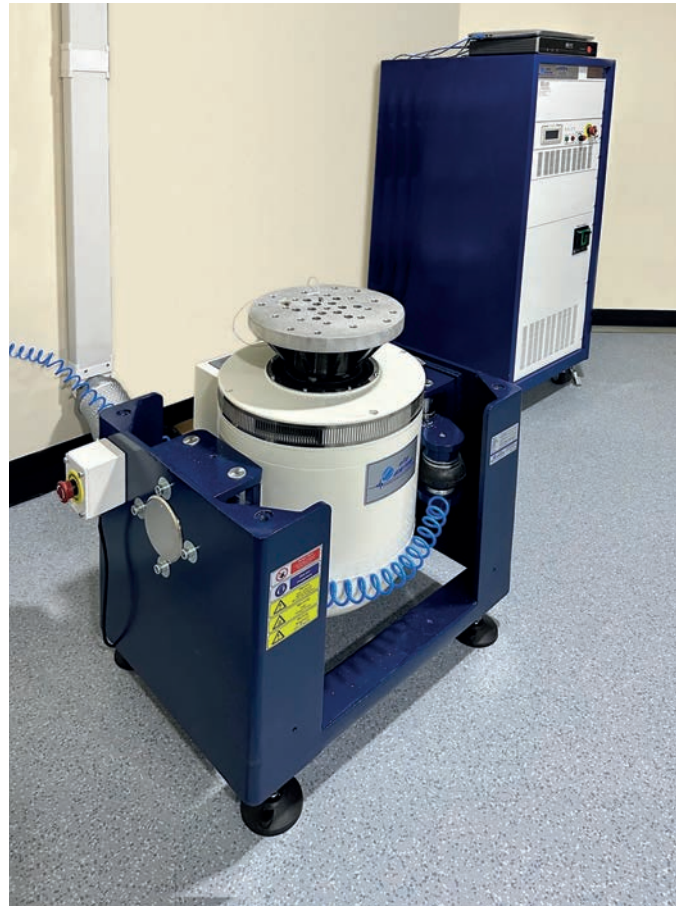
Specialist vibration / shock qualification testing equipment at Resolve Optics
