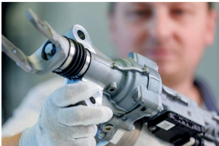
The new mechatronic rear-wheel steering system by Schaeffler has celebrated its series-production premiere, bringing enhanced agility on bends and superior inner-city maneuverability to the new electric SUV of a leading international car manufacturer
