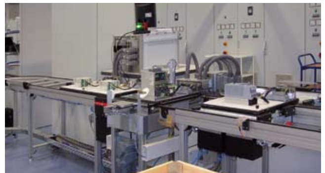
Automatic high voltage testing system
