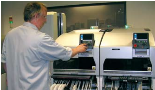
High speed SMD assembly plant
