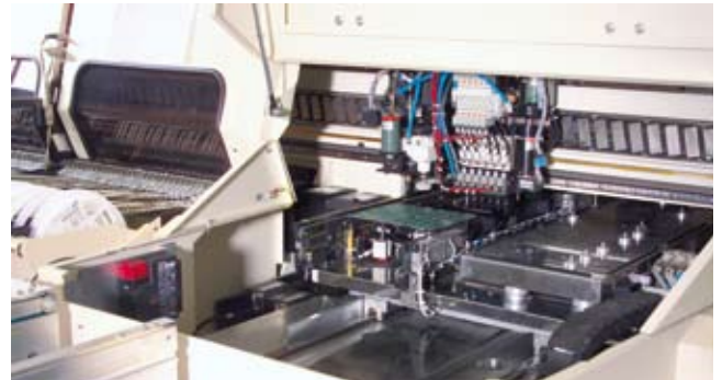
Automatic assembly of circuit boards
