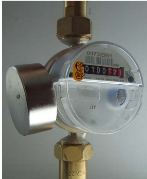
Fig. 5. Neodymium magnet left on the water meter by a 'forgetful' water consumer; the photo was taken during a reading by an inspector (the authors received this photo from one of water utilities)
