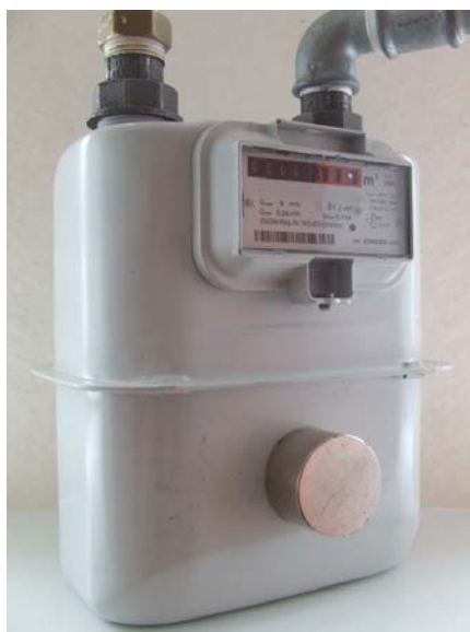
Fig. 3. Attack with neodymium magnet on gas meter diaphragm
