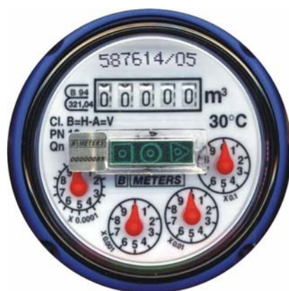
Fig. 9. Magnetic field indicator MFI-3 installed on a water meter [16]
