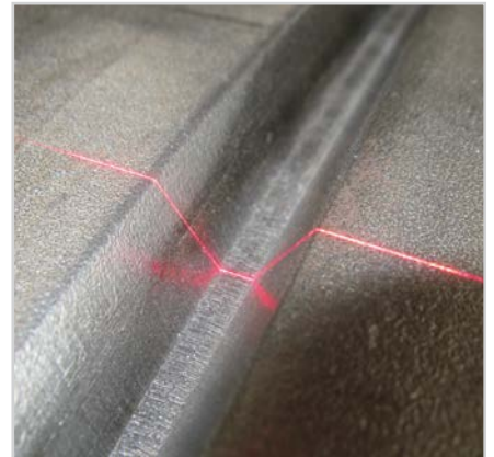
V-gap measurement on pipes
