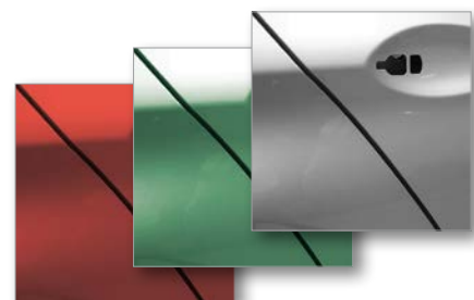
Auto exposure is important for measurements with changing surfaces
