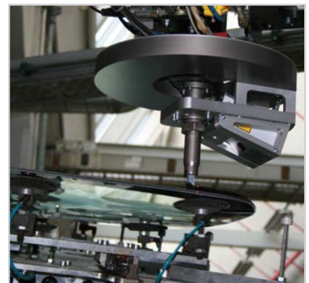
Inspection of the adhesive beading
